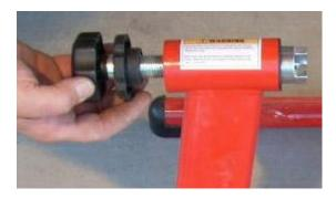
6. Insert the axle end first that does not have the handle on it as shown below.
