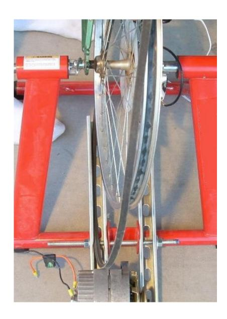
7. Connect the loose rubber band to the mini rotor on the base of the stand.
