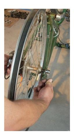
4. Make sure the wheel is equidistant from the frame. This is a very common mistake. Notice in the picture below how the gaps between each side of the wheel and frame are the same size. You need to do the same comparison check.
