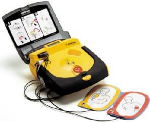
*It is a portable electronic device that automatically diagnoses the life-threatening cardiac fibrillation, and is able to apply electrical therapy, helping the heart to regain an effective rhythm.*
