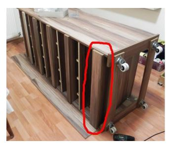
For the back stoppers, you'll use only 4x31-inch boards using exactly the same method.
