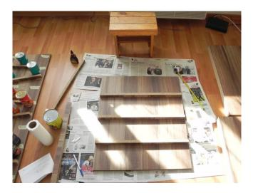
First, you'll need to divide the board into three to six equal parts, depending on what module you are building. Then draw a line on every side of the delimiter.
