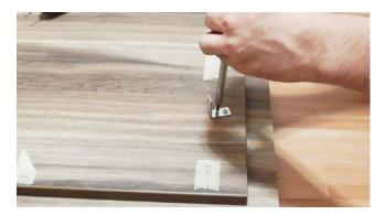
With one hand, hold the board, and with the other one, mark the place where you need to drill.
