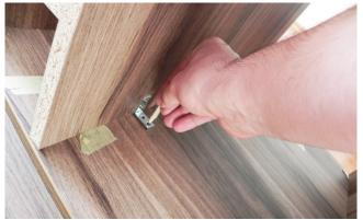
Push the board a little bit behind so you can drill the holes, both below and above. (In the image, you can see the holes I drilled in the big board below.)
