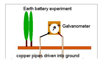
If you want to try it then get two copper rods or pipe and drive them into the ground and then connect a galvanometer(place them near a tree for better results.) apparently the needle always points positive although it may take time for the current and voltage to build up.
