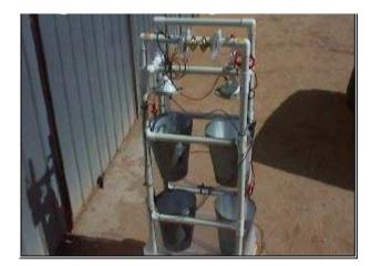
front view of author's unit notice the brass door knobs used as a spark gap.
