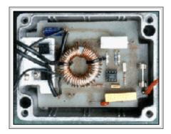
The step up converter built from a kit. It starts from just four volts snd outputs s regulated 14 volts to the battery
