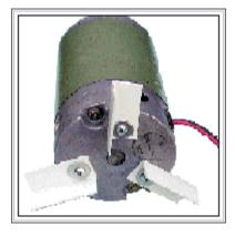
This rear view shows the three plastic angle sections used to make the motor a tight fit in the mast
