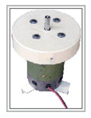
The DC motor fitted to the plastic end cap which holds it to the mast
