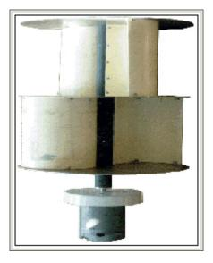
Here you can see the whole motor and rotor assembly before fitting to the mast and painting. Note how the vanes in the top section are rotated 90 to those in the bottom section and the motor does not yet have the plastic angle sections attached.
