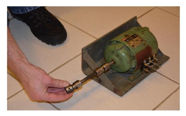
The connection between the two can be either direct (like the one we are doing) or a pulleys and belts system (here you have below another model that can be fit to this project if you have that type of connection on the air pump):
