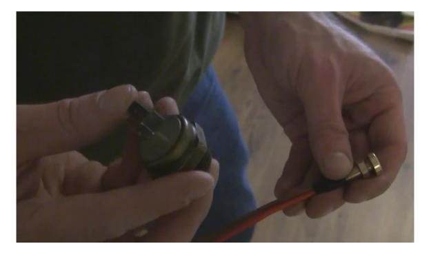
This sensor will actually cut the power supply for the air pump anytime the pressure inside the container will reach the proper pressure. It's best to fasten the sensor very well to make sure the recipient is pressurized.
