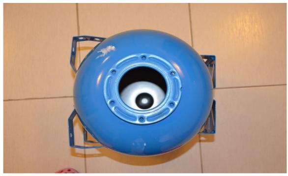
We will place the container on the holder so that one of the ends (where we will place the pressure sensor) will reach the edge of the holder and the other end we will leave a larger space where we will connect the pipes to the air pump. We will also leave about 3 inches distance from the edge of the holder.
