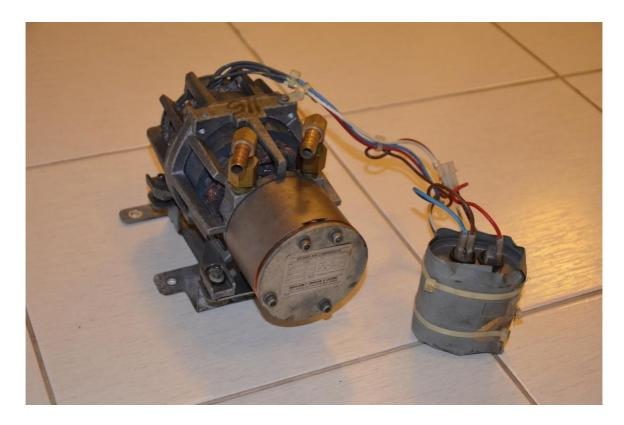
The air pump has 2 ways for the air circuit, a supply cable and a capacitor for turning on the circuit on its own. The air pump can be taken from any air compression system, medical devices, air conditioner systems etc.
