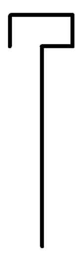
(The shape used for the iron bar which connects the generator to the ground) This should be about 1.5 - 2.0 feet long. Also you have to drill some holes into the handle in order to attach the copper wire from the generator.
