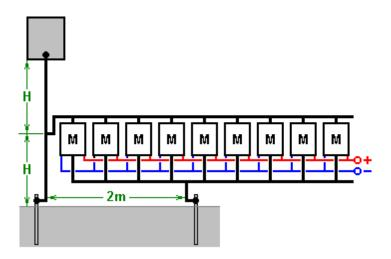
With this arrangement a single module produces around 30 volts while the original method of connecting near the earth was giving about 26 volts with two modules.
