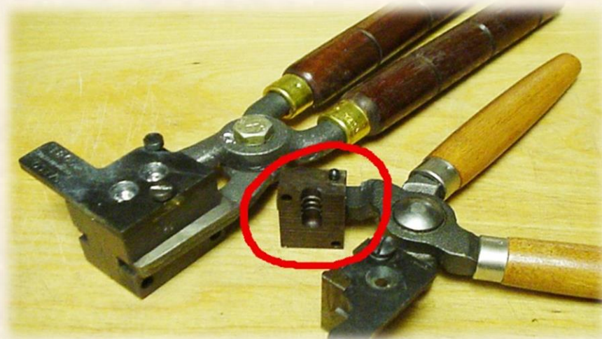
(Two bullet molds. The single cavity mold is open and empty. The double cavity mold is closed and contains two bullets. Photo Credits: Thewellman)
