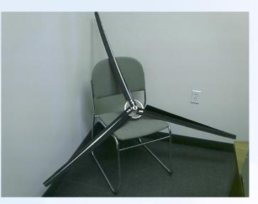
ABS or PVC. I have also heard that green sewer pipe that is 3/8" thick makes great blades that are durable. If you want to do nice ones, I recommend making out of fiberglass, much stronger. I would make a simple mold and use a foam core, use about 6-10 layers of woven glass.
