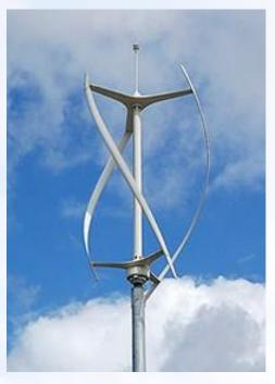
With a vertical axis, the generator and other primary components can be placed near the ground, so the tower does not
