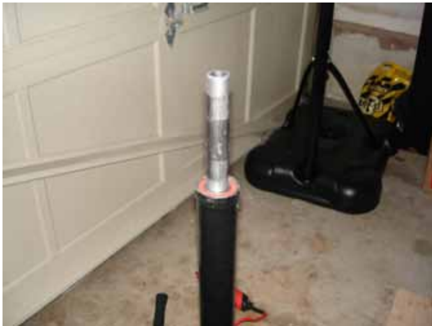
A fully assembled Yaw System
